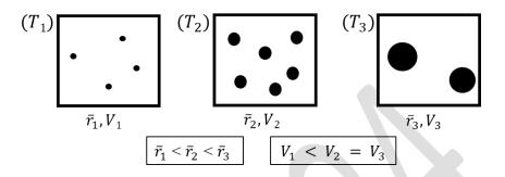
If the cementite in steel is more noble than ferrite, then which one of the three microstructures will have the highest corrosion rate when exposed to an aqueous solution of 3.5 wt. % NaCl?
